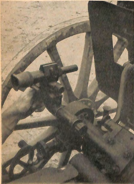
(Above) Figure 290. Telescopic sight for model 92 (1932) 7.7-mm machine gun has a 4 × magnification, a 10° field of view, and a weight of 3 lbs., 6 ozs.
